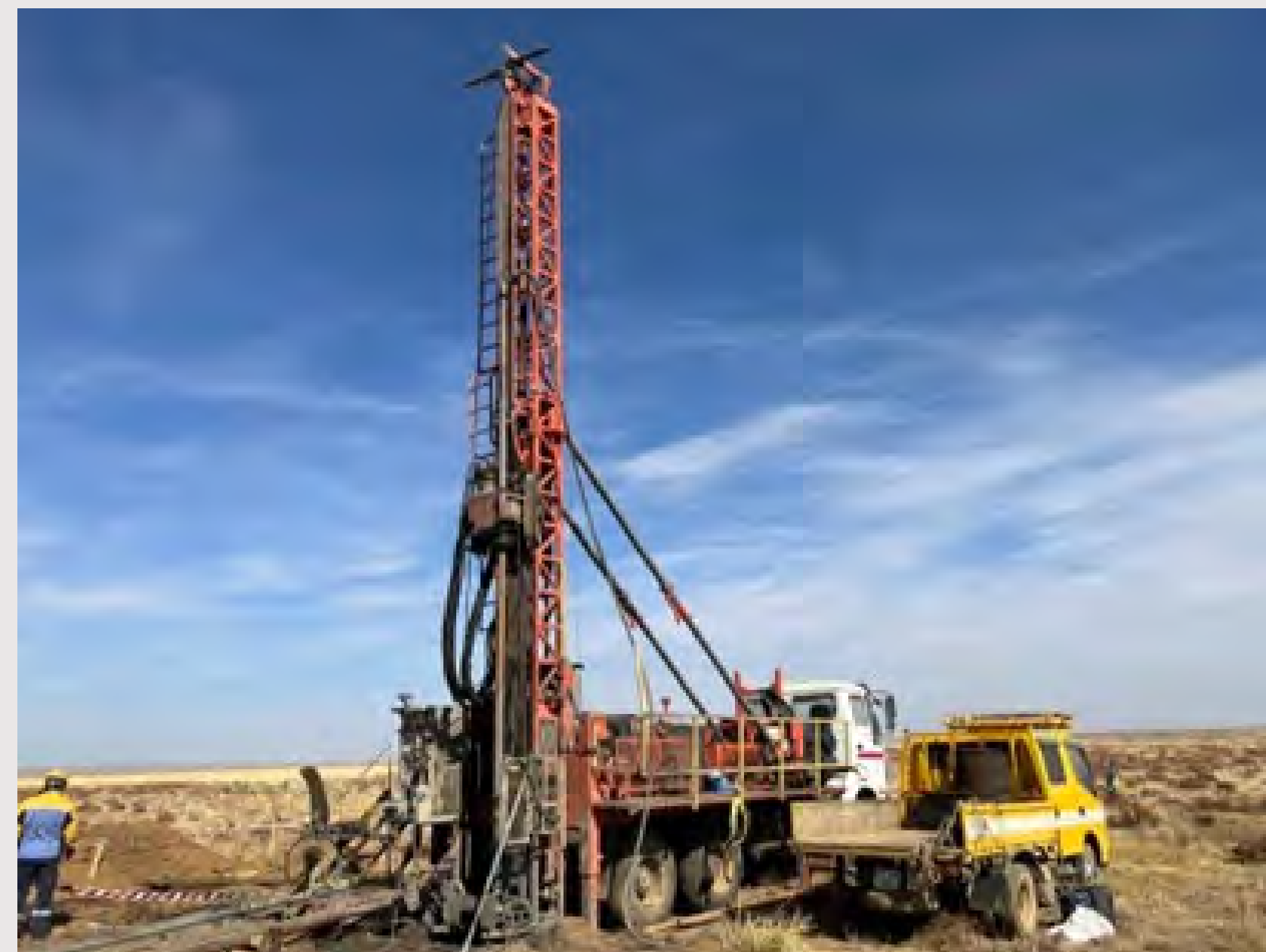
Diamond core drilling at UNDH-02
